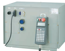
AR21 PW controller • Power up (1.3KW, 1.8KW) 540×360×400 28kg • 3 phase AC200/220V
