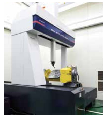
Accuracy measurement with large 3 Dimensional Measuring Machine
