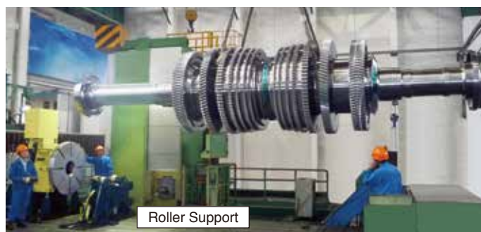
Simultaneous 3 axes control of X, Z & A axis
