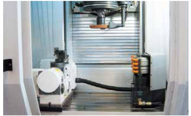
5AX-150 for 4th and 5th axes tilting rotary table on special grinding center
