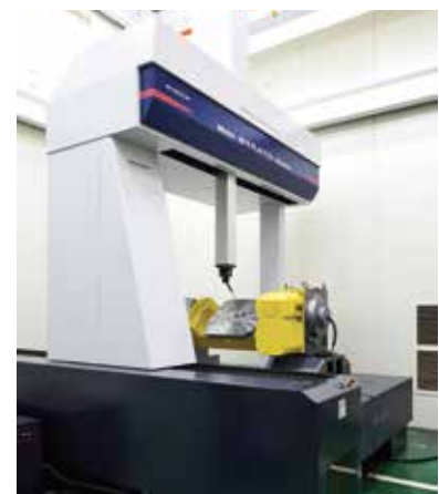
Accuracy measurement with large 3 Dimensional Measuring Machine
