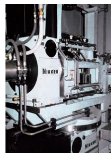
CNC401T is installed on CNC600.
