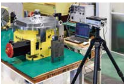
Indexing Accuracy Measurement by Laser
