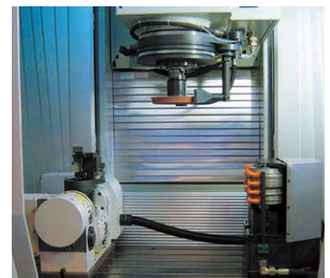
Utilization for 4th and 5th axis rotary table of special grinding center
