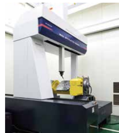
Accuracy measurement with large 3 Dimensional Measuring Machine
