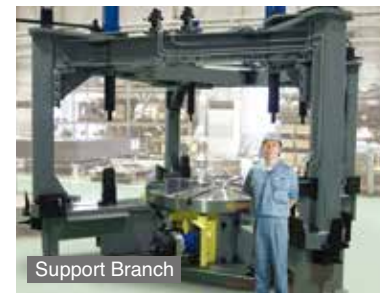
CNC1800 & Support Branch Indexing/ clamping of the turbine disk
