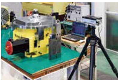
Indexing Accuracy Measurement by Laser
