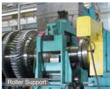
Simultaneous 3 axes control of X, Z & A axis
