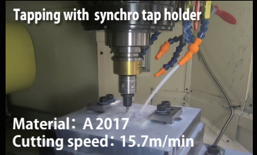
Tapping with the synchro tap holder with the fine floating (M6)
