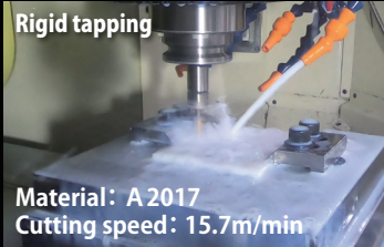
Tapping with the synchro tap holder with the fine floating (M6)
