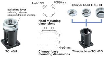
Please use the TCL-GH clamper as a clamper for tools that do not have drive grooves or U grooves, such as the HSK E / F type. Different shanks canbe clamped as long as the V-flange diameter is the same.
